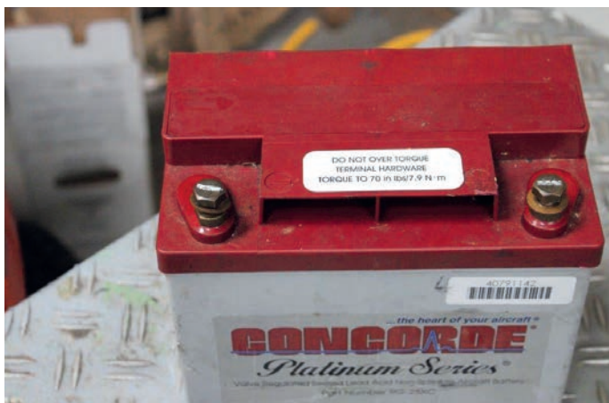
Figure 1: Inspect the battery terminals for signs of corrosion and security
