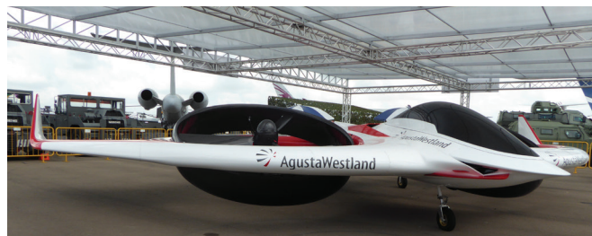
AgustaWestland exhibited its Project Zero electric tiltrotor demonstrator at the Singapore Airshow in February. The aircraft can at present only fly for 10 minutes but this will increase, says the company, which is also working on a diesel hybrid version that could fly for an hour.
