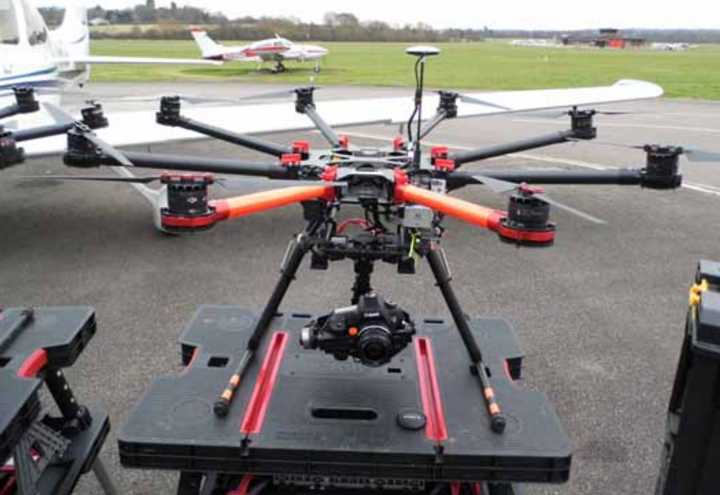
A DJI S1000 fully kitted out costs around £8,000. These larger drones are flown by the pilot with one controller and a separate video control unit for the cameraman/look-out.
