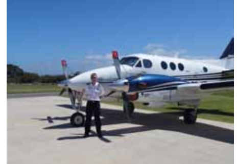
Advanced instructor Michael Haasbroek is qualified to teach cadets to fly the King Air C90. One of AIFA's King Airs (pictured) has modern Garmin G600 avionics and a Blackhawk PT-6 engine performance upgrade, while the other two "may be getting a full avionics upgrade."
