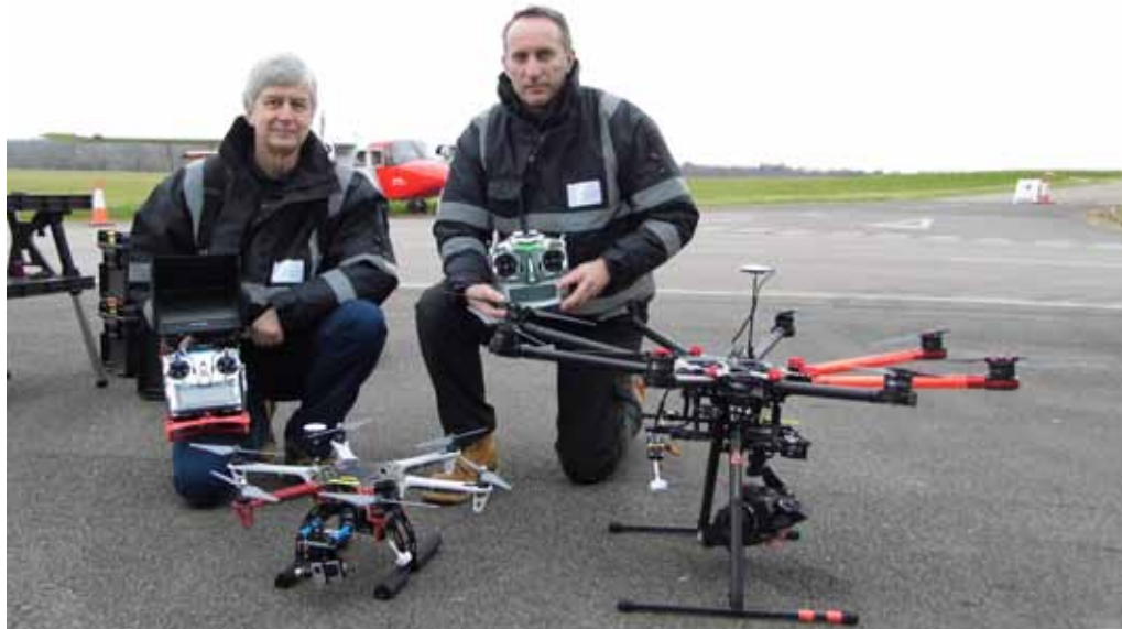
The current iSkyUAV fleet consists of Huey (F550), plus the larger Louie and Dewey (pictured) S1000 models. The company also has specialist drones and has the engineering skills to tailor drones for particular missions.
