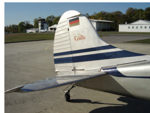
Left: clamshell cowling make for easy access to the Rolls Royce Continental Above: beautifully proportioned Art Deco tailplane looks better than that of the C172 Below: tail wheel assembly allows some directional control during taxiing
