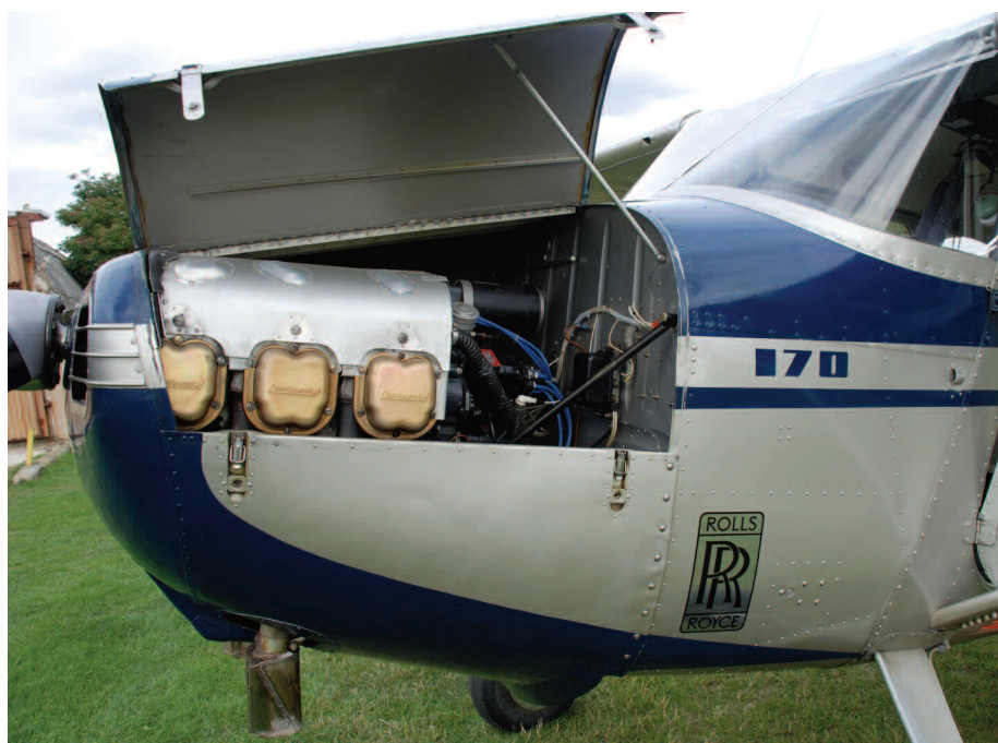
Left: clamshell cowling make for easy access to the Rolls Royce Continental Above: beautifully proportioned Art Deco tailplane looks better than that of the C172 Below: tail wheel assembly allows some directional control during taxiing
