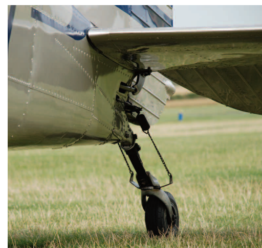
Left: clamshell cowling make for easy access to the Rolls Royce Continental Above: beautifully proportioned Art Deco tailplane looks better than that of the C172 Below: tail wheel assembly allows some directional control during taxiing
