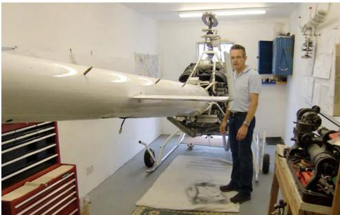
torque links, fuel pumps, hoses and clamps, flight and engine instruments, wiring loom, and bill. Finally you get the main rotor blades, engine and fadec system, and you're off to the races. RotorWay makes its own engine, a four cylinder, horizontally opposed, fuel injected, water cooled 2.7 litre unit producing 150 to 170 horsepower, depending on who you listen to, on premium unleaded. You can use avgas, but if you do the TBO comes down because it causes lead fouling and other problems.
