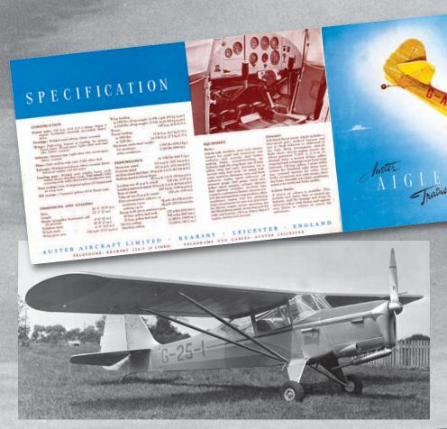
Left: the prototype Aiglet Trainer, an Autocrat fuselage married to a 130 hp engine Above: the brochure model, G-AMMS, is still in flying condition today Main picture: shorter wings and larger tail marked out the Trainer
