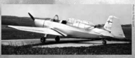
Left: the Zlin was flown solo from the rear seat and could not be started from the front Above: Zlin 126 – the only visible difference from the 226 was the lack of a tow hook Below: OK-JEB, the Zlin Trener 6 used by the author for this flight test in 1956
