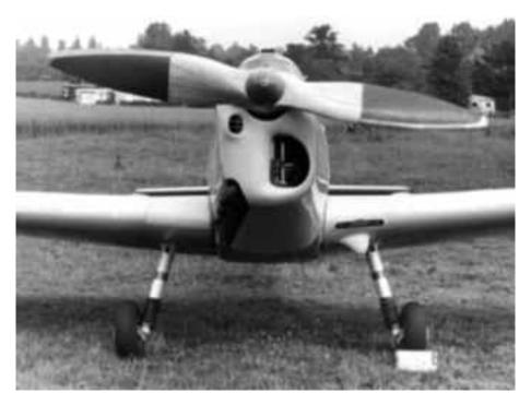
steerable tailwheel doing most of the work. Take-off acceleration was rapid, with 160 horses pulling 818kg (1800lbs) quickly into the air. Following an unstick at about 85km/hr (53mph) the Zlin of the time was soon at the recommended climb speed of 120 (75) with a surprisingly nose-up angle producing a very creditable 1350 feet per minute.
