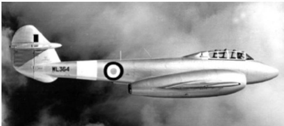
Left: the two-seat Mk 7 was the first Meteor dual trainer; previously all flights were solo Below left: slow throttle response caught out many Meteor pilots used to piston power
