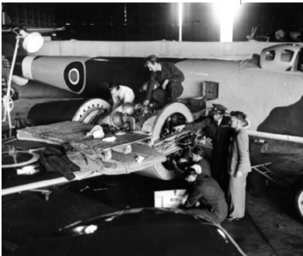
Left: RAF High Speed Flight engineers at Tangmere prepare the Rolls Royce Derwent 5 of Group Captain E.M. Donaldson's speed-record setting Meteor F4 in 1946
