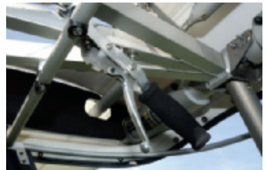
Left: rear fuselage structure is composite on aluminium framework Above: the oddest feature at first acquaintance is the centre stick, but it has many advantages Right: manual flap lever is above your head Below: best cruise speed is around 82 kt, and she can be trimmed to fly hands-off Bottom: deceleration is rapid when you cut the power and can catch out the unwary
