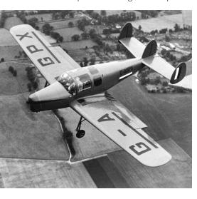
1800 rpm. Taking it further down the scale, slight buffet begins at just over 50 mph and the published clean stall occurs at a reduction of a further 12. The breakaway behaviour is benign.
