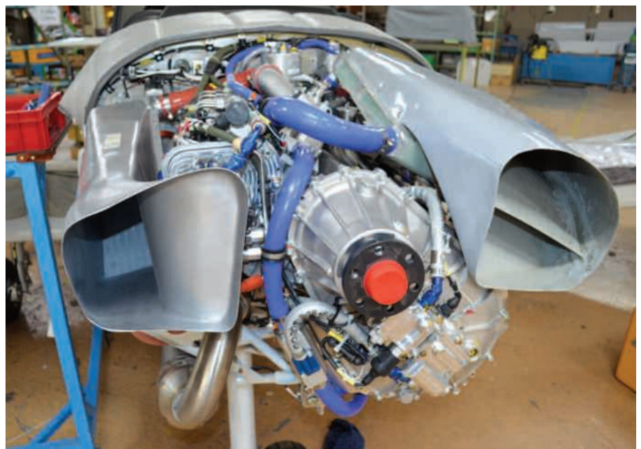
Above: two big air ducts cool the turbo (left side) and the cylinders equally Right: by contrast, the Lycoming takes up relatively little room under the cowling Below: silencer can allow the EcoFlyer to go anywhere, even in Germany
