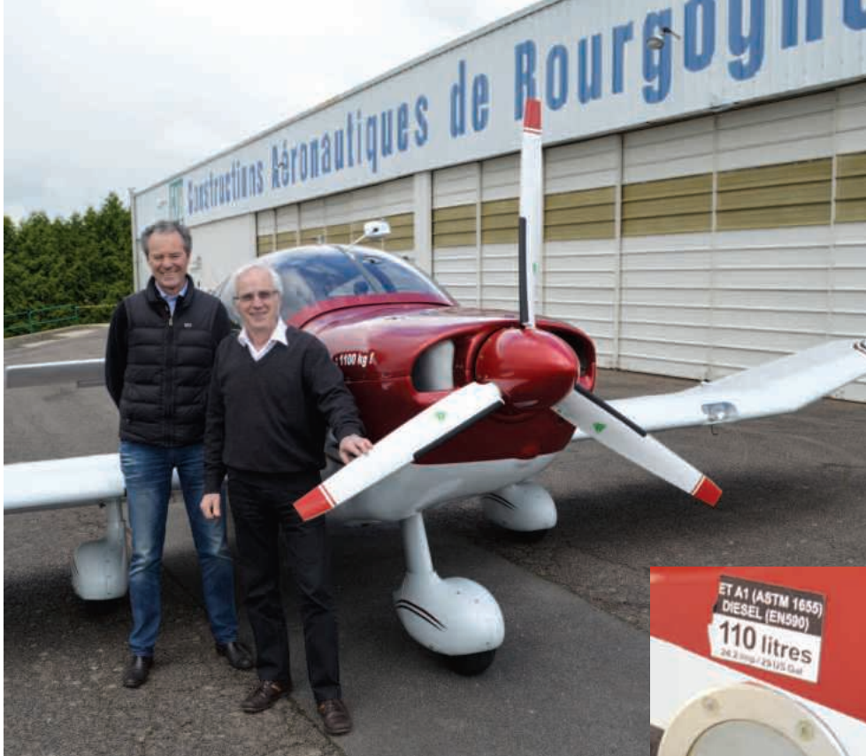
Above: Guy Pellissier and Daniel Triques, principals of Robin New Aircraft, with the EcoFlyer Right: no avgas here – the EcoFlyer's main tank filler is placarded for JetA1 Far right: weight shift – Robin makes much of the carrying capacity of the EcoFlyer
