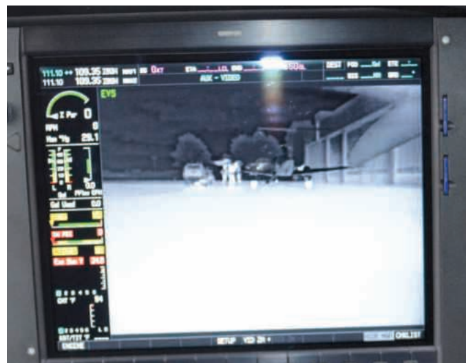
Above left: engine status information selected on the Multi-Function Display Above right: night vision system is useful on approach to low-light airfields Left: control panel, with the fabled 'blue button' in the centre
