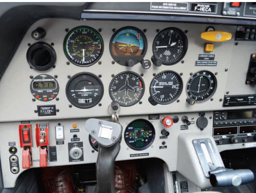
Above: EcoFlyer panel, with single power lever – yellow handle is for glider release
