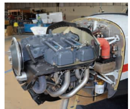
Above: two big air ducts cool the turbo (left side) and the cylinders equally Right: by contrast, the Lycoming takes up relatively little room under the cowling Below: silencer can allow the EcoFlyer to go anywhere, even in Germany
