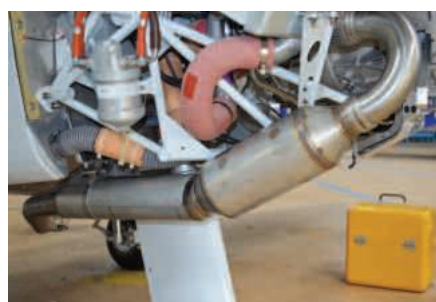
Above: two big air ducts cool the turbo (left side) and the cylinders equally Right: by contrast, the Lycoming takes up relatively little room under the cowling Below: silencer can allow the EcoFlyer to go anywhere, even in Germany
